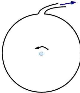
Figure 5: an aeolipile with an exhaust nozzle shaped like the space between two conventional turbine blades. Covering the outer perimeter of the aeolipile with these nozzles, a design similar to a conventional turbine results.
