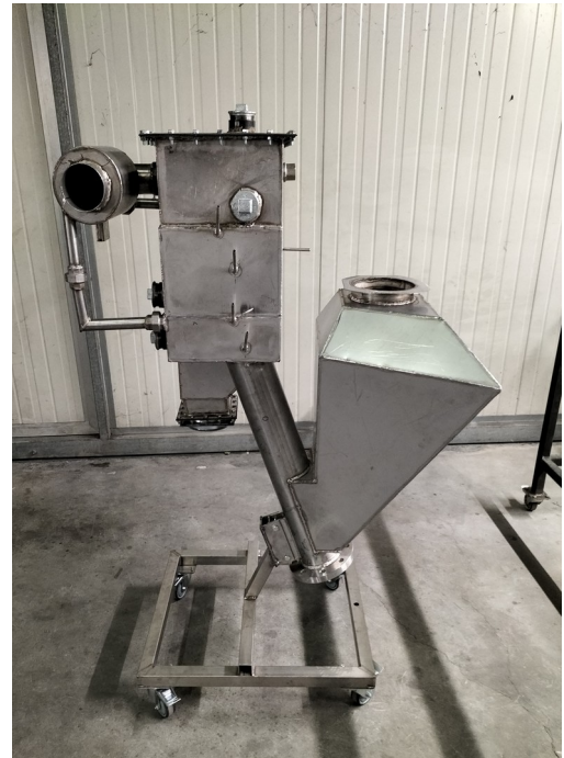
Figure 4: the gasifier, equipped with external burner (to the left) and preheating system for primary air.
